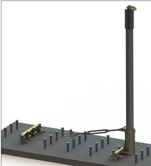
FIGURE 6: SINGLE POINT ANCHORAGE
