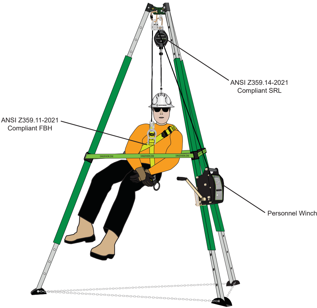
FIGURE 11 - EXAMPLE SYSTEM CONNECTIONS
